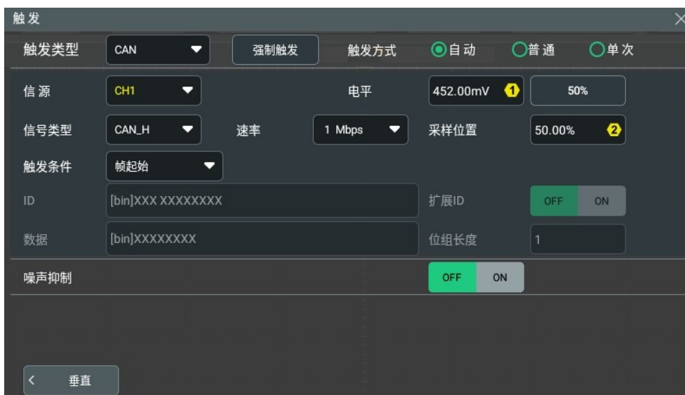
图 8.33 CAN 触发配置菜单
