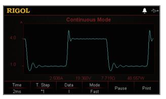
The electronic load provides the waveform display function and supports the following operations for the waveform, such as pausing the waveform, recording the waveform, and capturing the waveform. Therefore, you can dynamically observe the trend of parameters changes.
