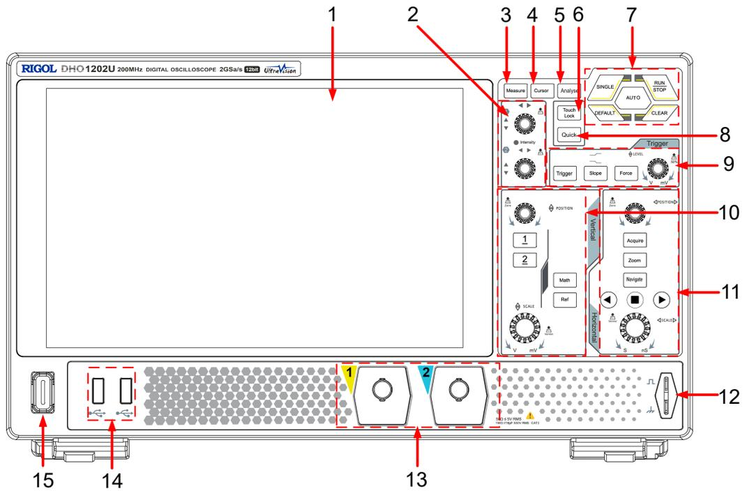
**Figure 4.2 Front Panel (2-channel Model)**
