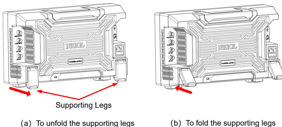
Figure 5.1 To Adjust the Supporting Legs
