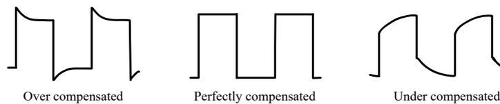
**Figure 5.6 Probe Compensation**
