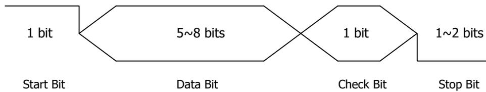
Figure 8.24 Schematic Diagram of RS232 Protocol
