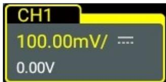
The information displayed in the channel status label is related to the current channel setting (irrelevant with the on/off status of the channel). After the channel is turned on, modify the parameters such as the vertical scale, horizontal time base, trigger mode, and trigger level according to the input signal for easy observation and measurement of the waveform.
