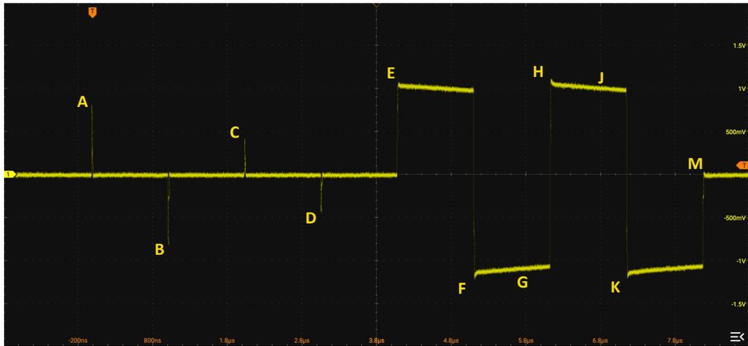
**Figure 20.4 Typical Waveform of Test Mode 1 Signal**
