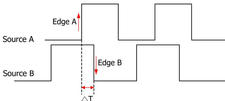
Figure 8.18 Delay Trigger
