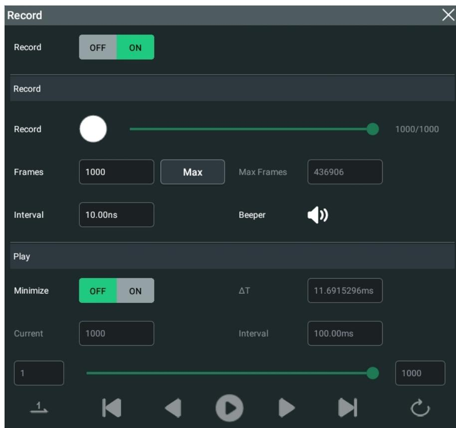
Figure 23.1 Waveform Recording Interface
