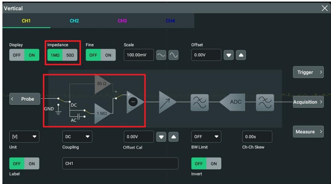
Figure 5.2 Input Impedance Modification
