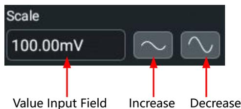
In the **Vertical** system menu, select **ON** or **OFF** to enable or disable the fine adjustment. By default, it is OFF. You can also press down the vertical scale knob on the small screen to enable or disable the fine adjustment.
