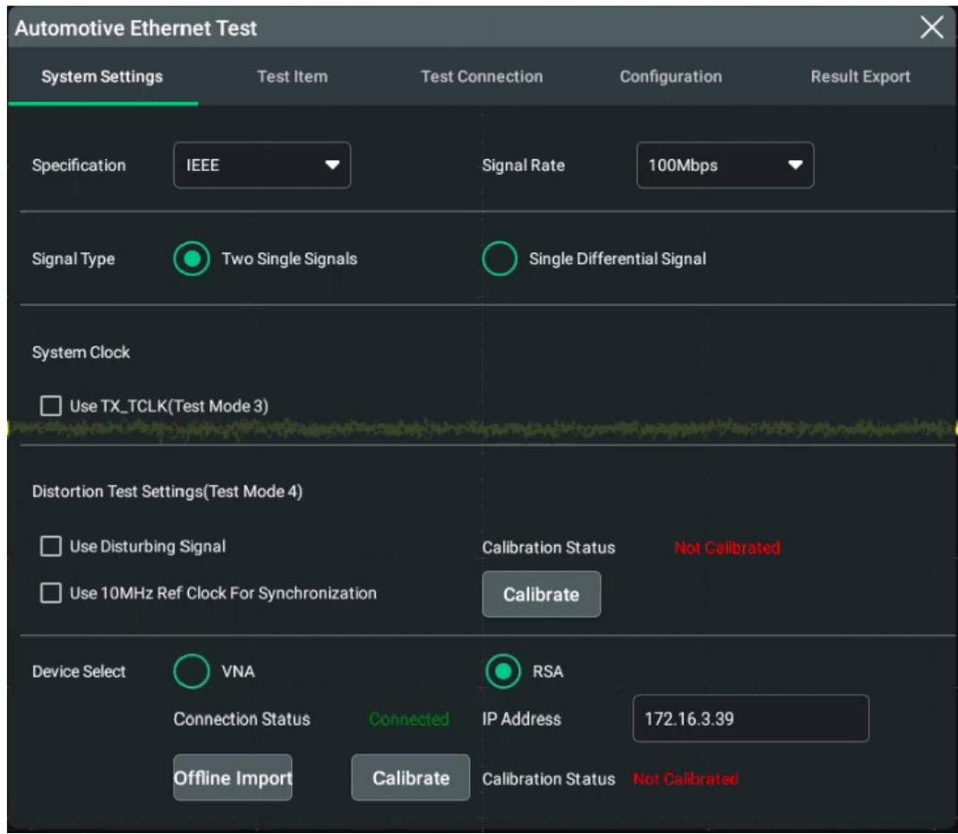
Figure 21.1 System Settings of the Automotive Ethernet Test
