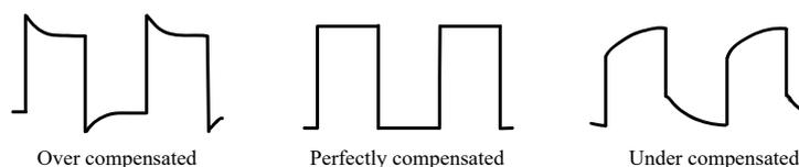
**Figure 4.9 Probe Compensation**
