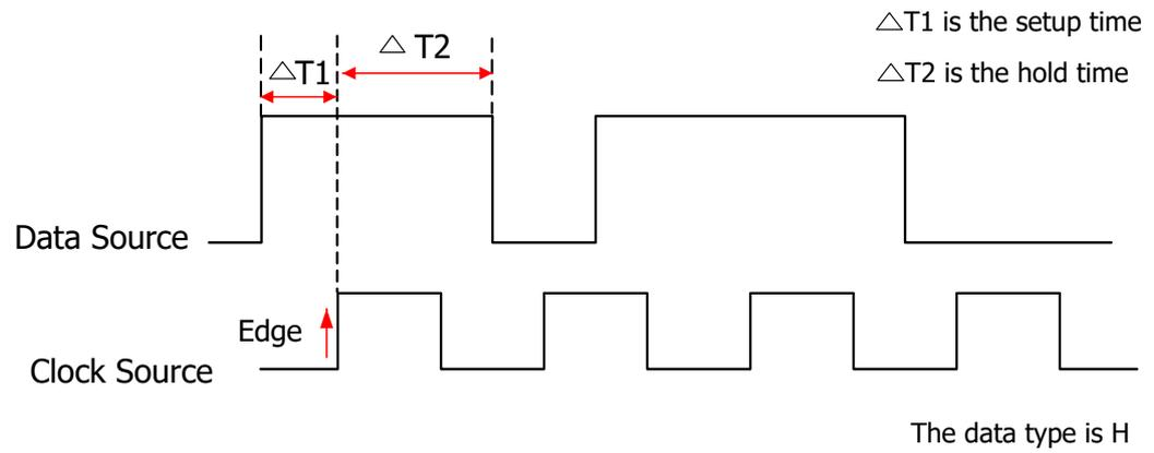
**Figure 8.20 Setup/Hold Trigger**
