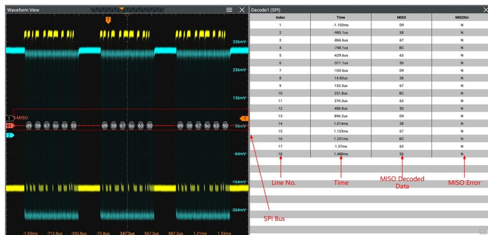
Figure 18.13 SPI Decoding Event Table
