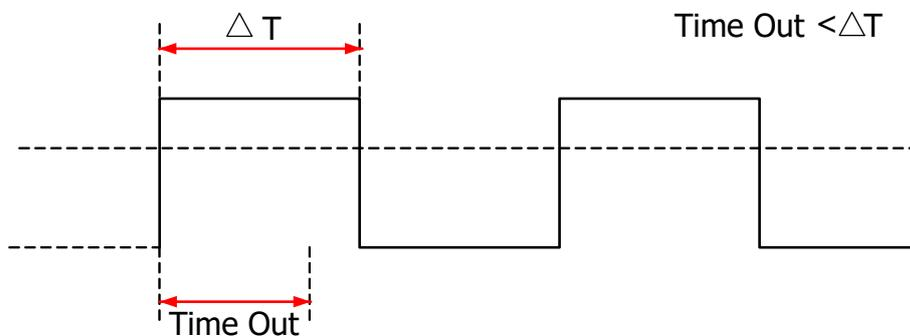
Figure 8.13 Timeout Trigger
