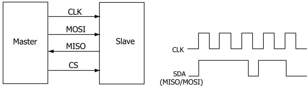
Figure 18.11 SPI Serial Bus
