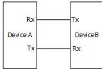
**Figure 18.4 Schematic Diagram of RS232 Serial Bus**
