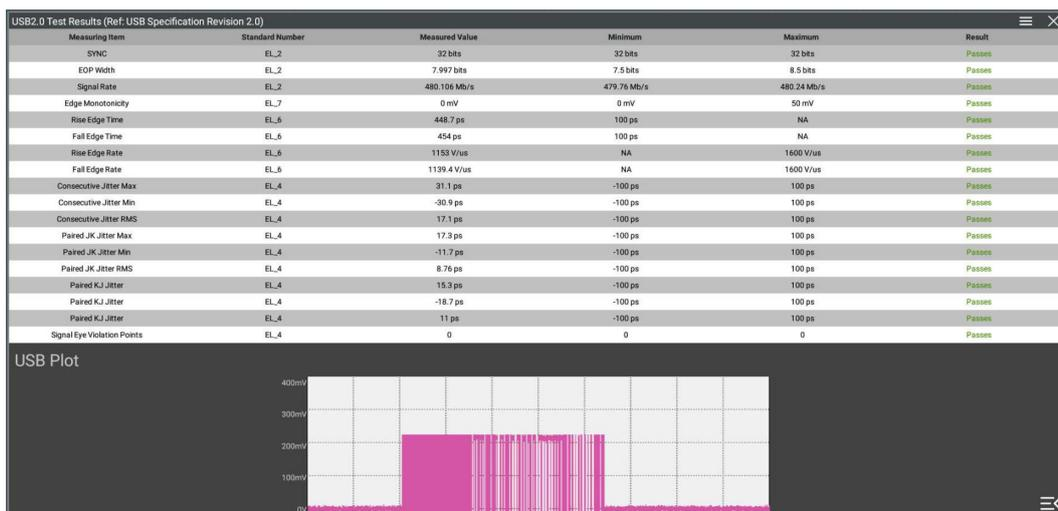
Figure 19.2 USB2.0 Signal Quality Compliance Analysis Test Result
