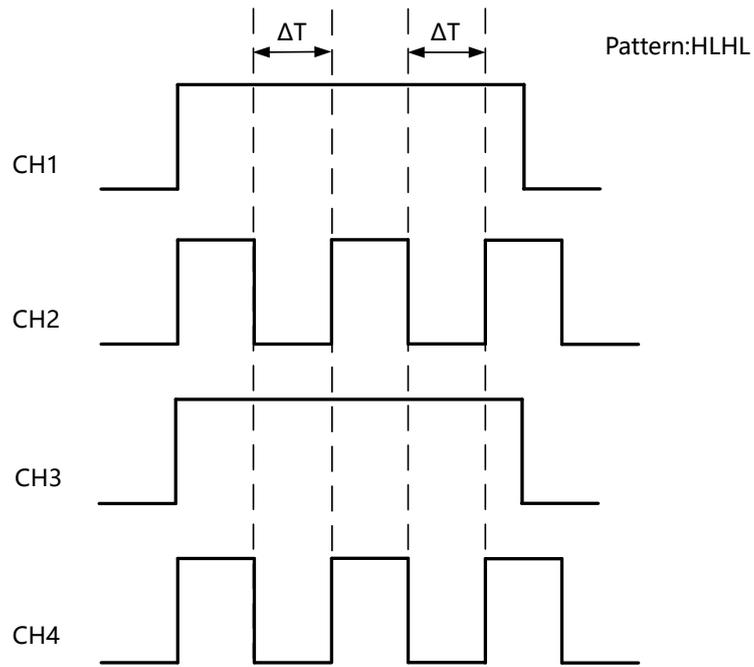
Figure 8.11 Duration Trigger
