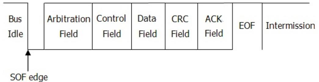
Figure 8.34 Data Frame Format of the CAN Bus
