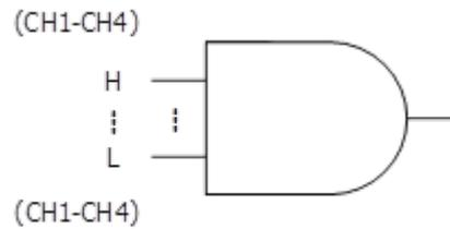
Figure 8.9 Pattern Trigger
