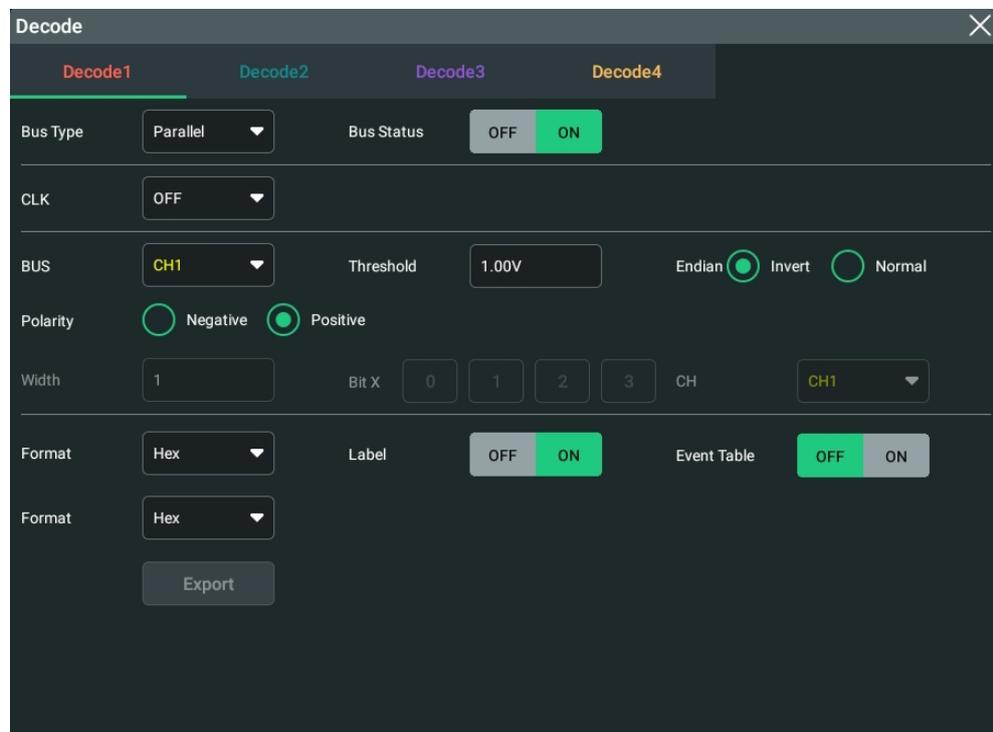
**Figure 18.2 Parallel Decoding Menu**
