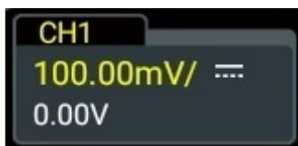
Click/tap the channel status label at the bottom of the screen or press the front-panel key
