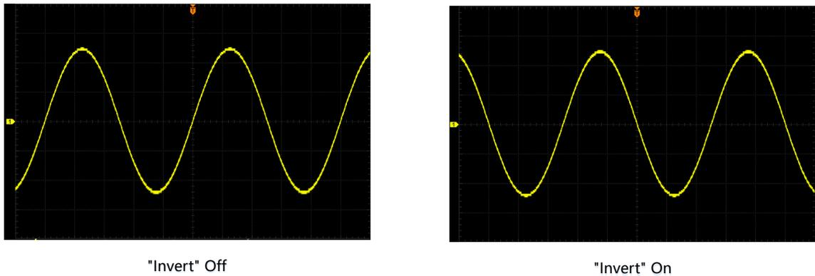
Figure 5.3 Waveform Invert
