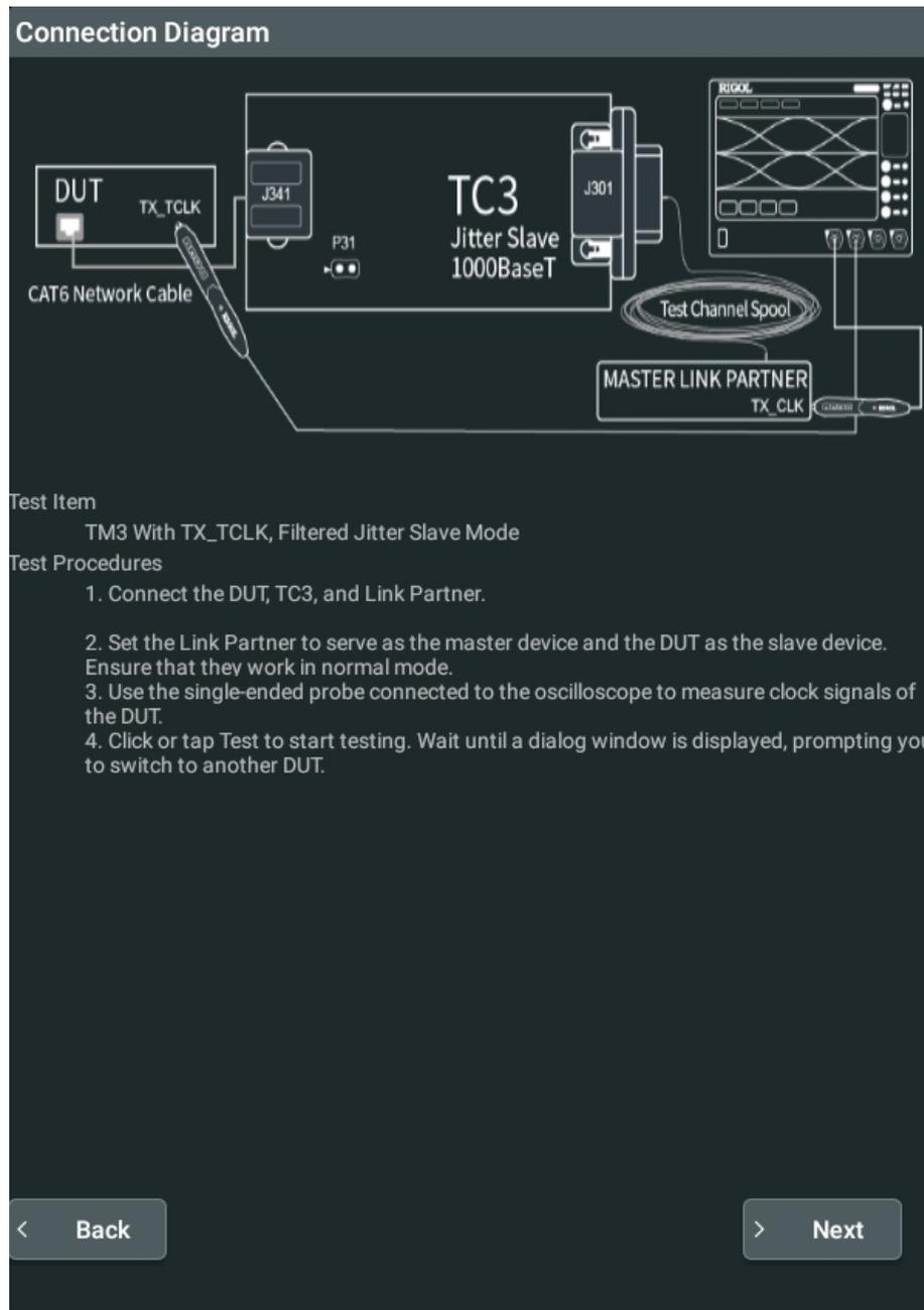
**Figure 20.6 Connection Diagram**
