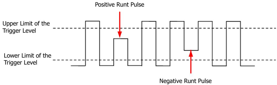
Figure 8.15 Runt Trigger
