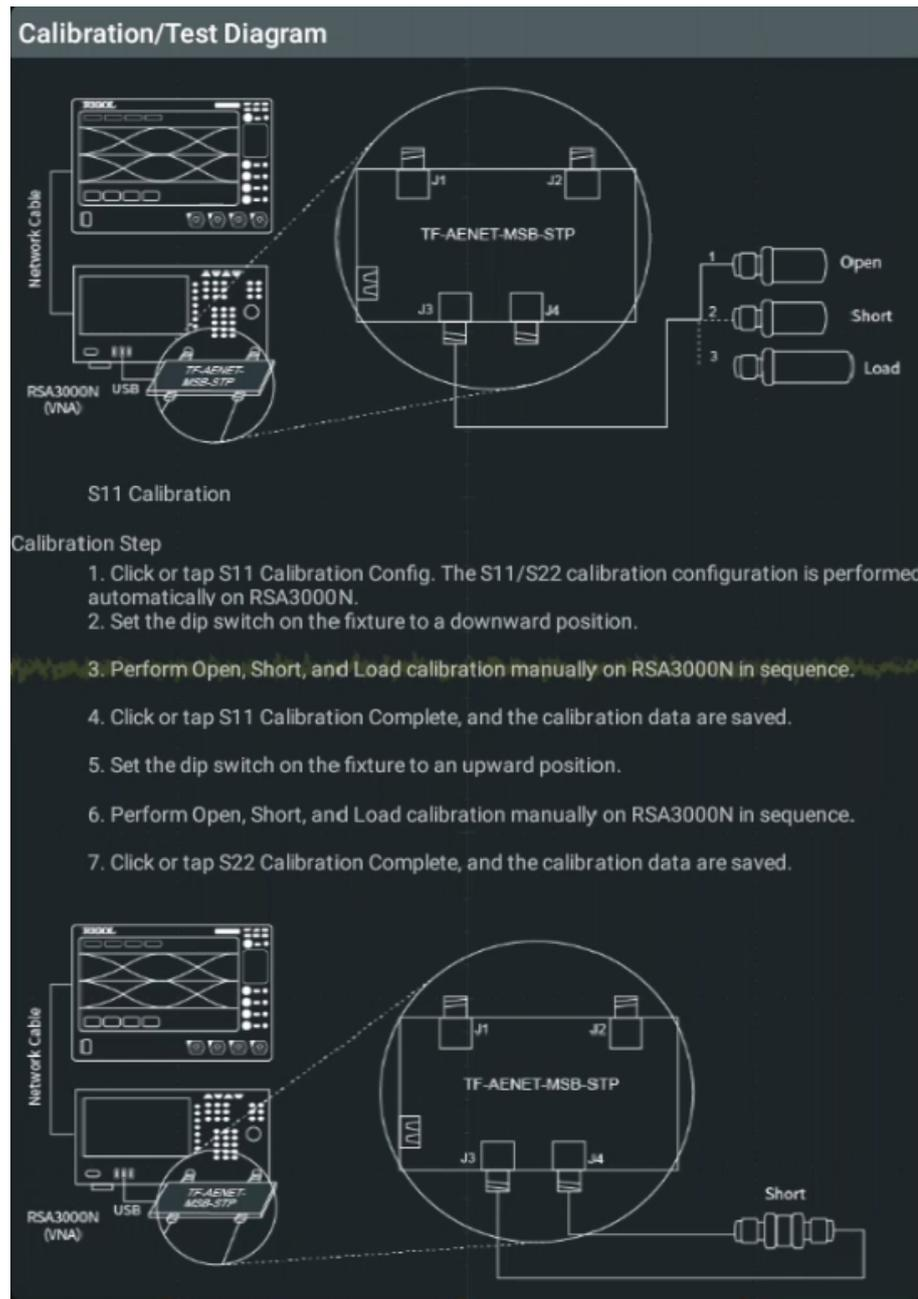
**Figure 21.4 Calibration Connection Diagram and Calibration Procedure**
