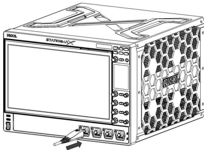
**Figure 4.6 Connect the Active Probe**
