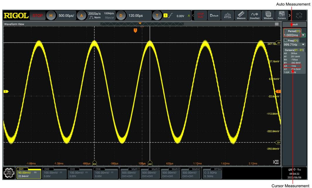
Figure 10.11 Manual Cursor Measurement Example
