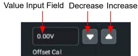
Its value is related to the input impedance and the vertical scale.
