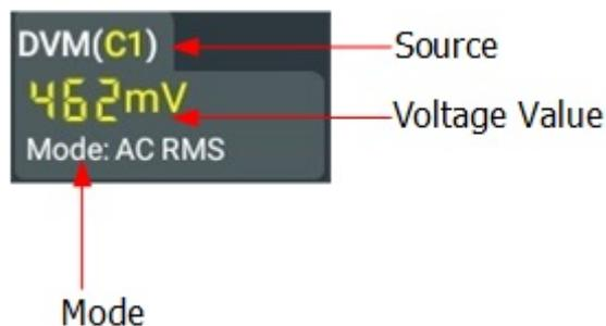
The specific value above shows the measurement extrema over the last 3 seconds.
