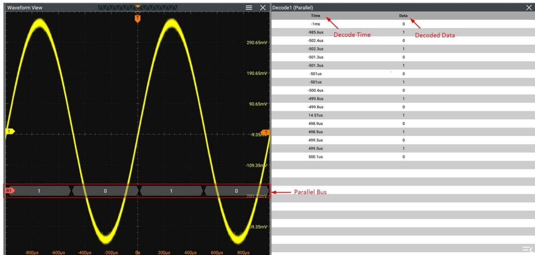
Figure 18.3 Parallel Decoding Event Table
