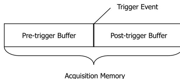
**Figure 8.1 Schematic Diagram of the Acquisition Memory**
