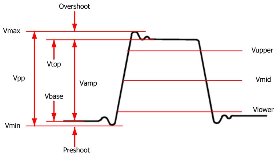
**Figure 10.3 Voltage Parameters**
