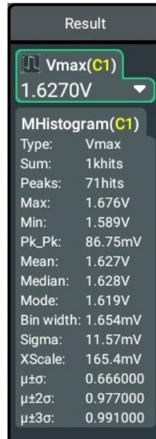
Figure 10.16 Measurement Histogram Result
