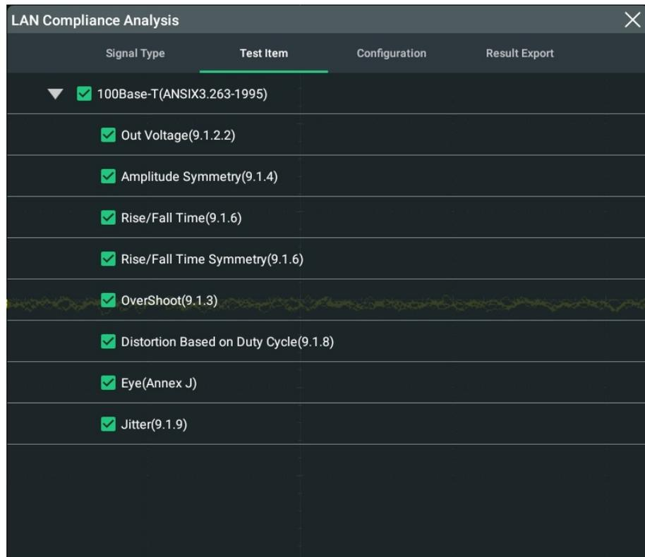
**Figure 20.2 100Base-T Signal Test Items**
