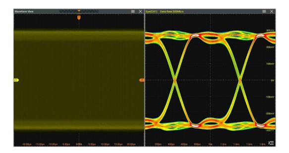
Figure 13.2 Eye Measurement Result
