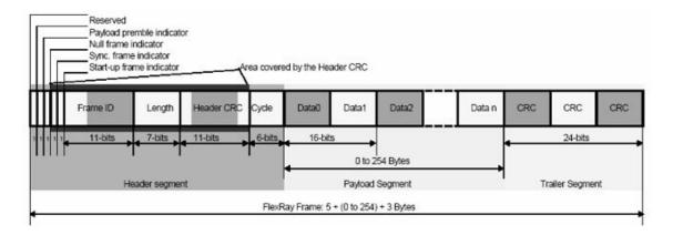
Figure 8.35 Frame Format of FlexRay Bus
