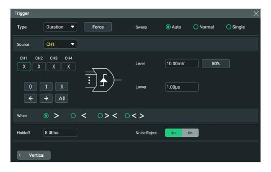
Figure 8.12 Duration Trigger Setting Menu
