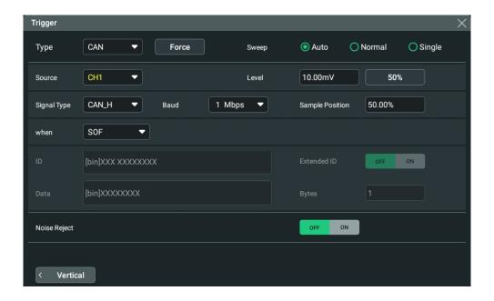
Figure 8.33 CAN Trigger Setting Menu
