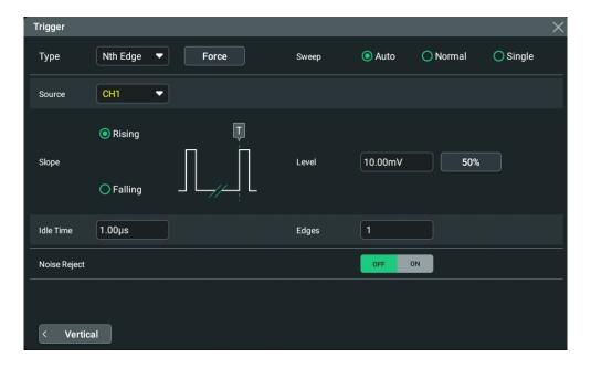
Figure 8.23 Nth Edge Trigger Setting Menu
