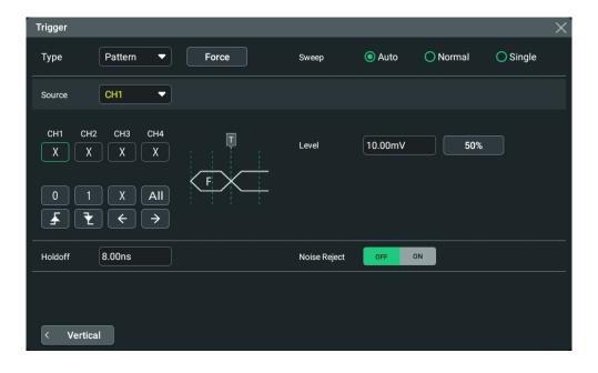
Figure 8.10 Pattern Trigger Setting Menu
