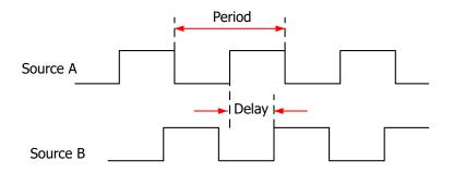
**Figure 10.2 Delay and Phase Parameters**
