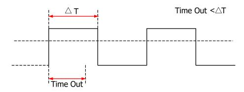
Figure 8.13 Timeout Trigger
