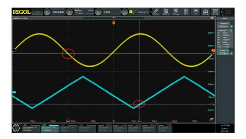
Figure 10.14 Track Measurement (after Horizontal Expansion)
