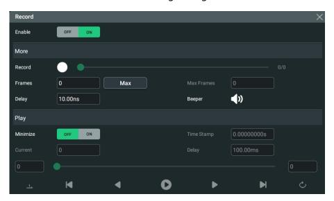
Figure 20.1 Waveform Recording Menu
