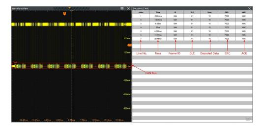
**Figure 17.18 CAN Decoding Event Table**
