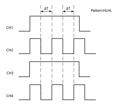
**Figure 8.11 Duration Trigger**
