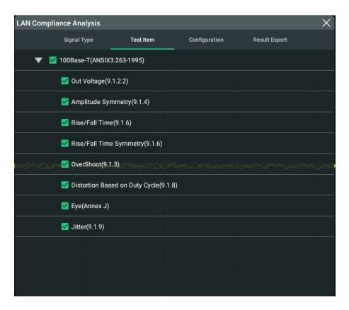
Figure 18.4 100Base-T Signal Test Items
