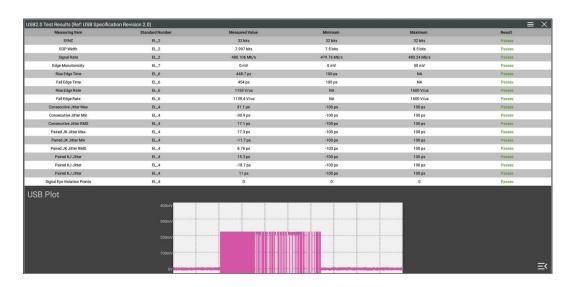
Figure 18.2 USB2.0 Signal Quality Compliance Analysis Test Result
