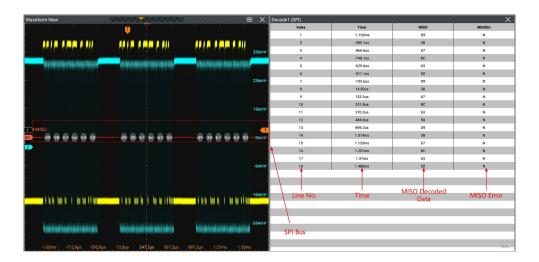
Figure 17.13 SPI Decoding Event Table
