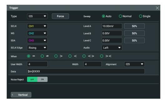
Figure 8.41 I2S Trigger Setting Menu
