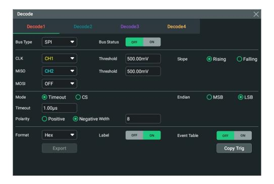
Figure 17.12 SPI Decoding Menu
