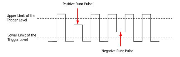
Figure 8.15 Runt Trigger
