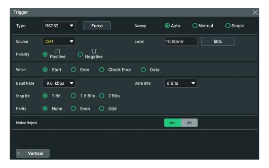
Figure 8.25 RS232 Trigger Setting Menu
