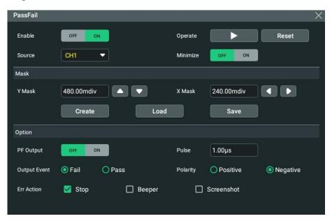
Figure 16.1 Pass/Fail Test Menu
