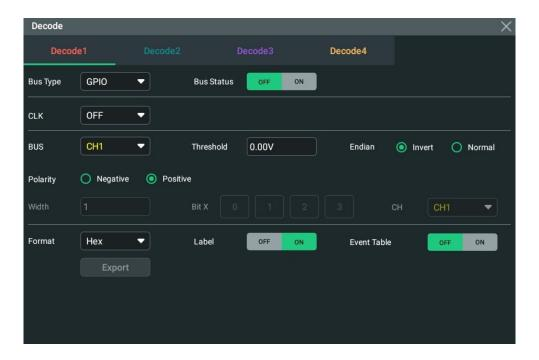
Figure 17.2 GPIO Decoding Menu
