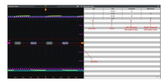
Figure 17.23 I2S Decoding Event Table
