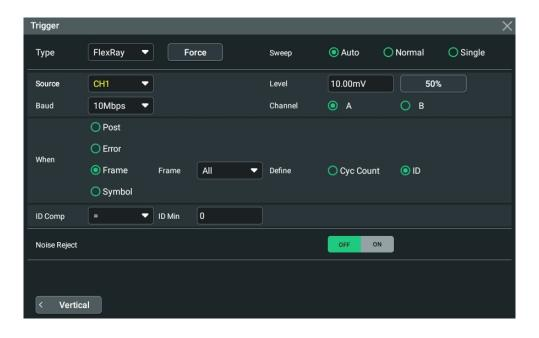
Figure 8.36 FlexRay Trigger Setting Menu
