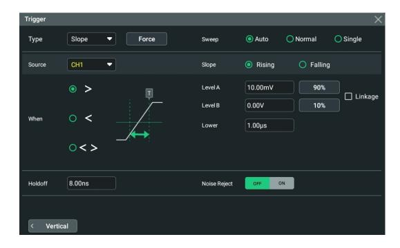
**Figure 8.7 Slope Trigger Setting Menu**
