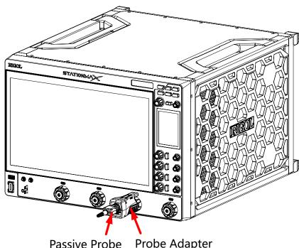
Passive Probe **Probe Adapter**
