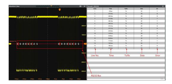
Figure 17.7 UART/RS232 Decoding Event Table
