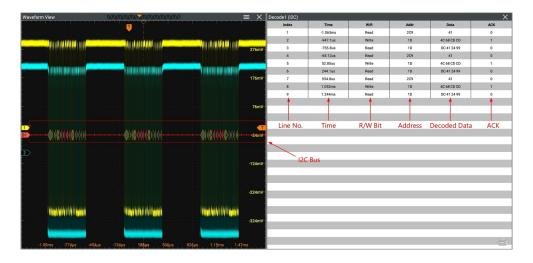
Figure 17.10 I2C Decoding Event Table
