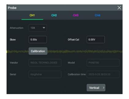
Figure 5.4 RP7000/PVA7000/PVA8000 Probe Setting Menu
