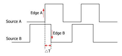
Figure 8.18 Delay Trigger
