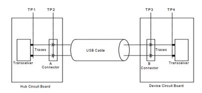
Figure 18.1 USB2.0 Test Model
