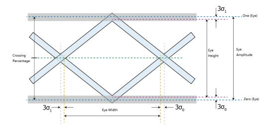
Figure 13.3 Diagram of Eye Measurement Parameters
