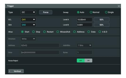
Figure 8.27 I2C Trigger Setting Menu
