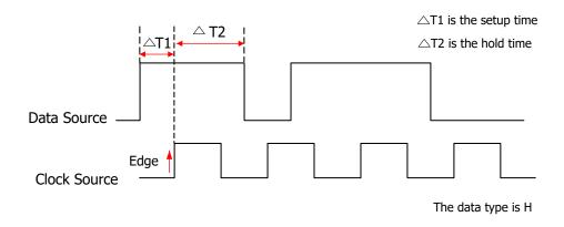
Figure 8.20 Setup/Hold Trigger
