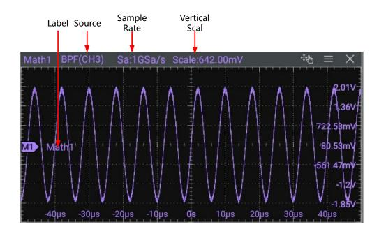
Figure 9.13 Operation Result Display Window
