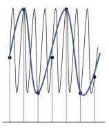
• **Waveform Leakage:** when the sample rate is too low, the waveform rebuilt from the sample data does not reflect all the actual signal information.
