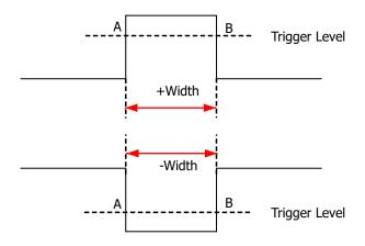
Figure 8.4 Positive Pulse Width/Negative Pulse Width
