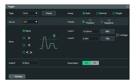
Figure 8.16 Runt Trigger Setting Menu
