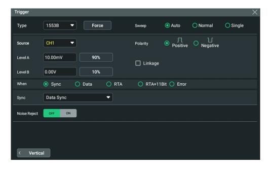
Figure 8.43 MIL-STD-1553 Trigger Setting Menu
