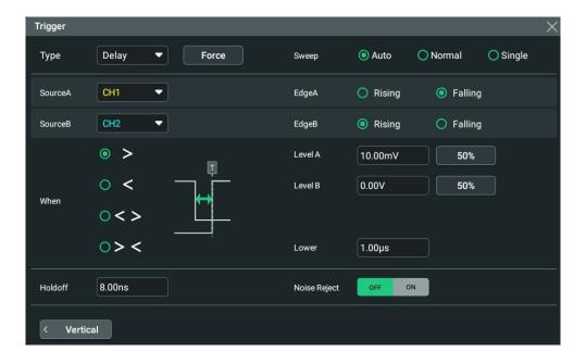
Figure 8.19 Delay Trigger Setting Menu
