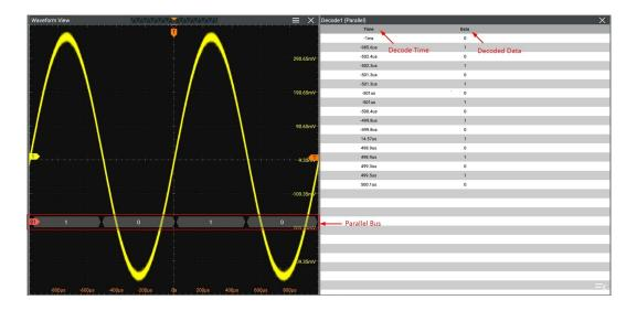
**Figure 17.3 Parallel Decoding Event Table**
