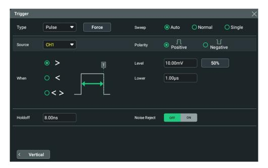
**Figure 8.5 Pulse Trigger Setting Menu**
