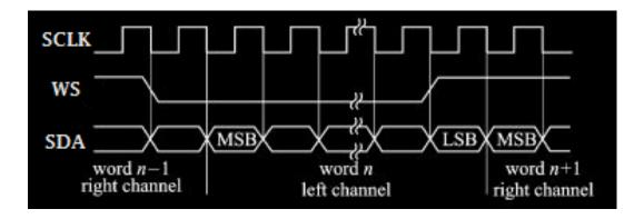
Figure 8.40 Sequential Chart of I2S Bus
