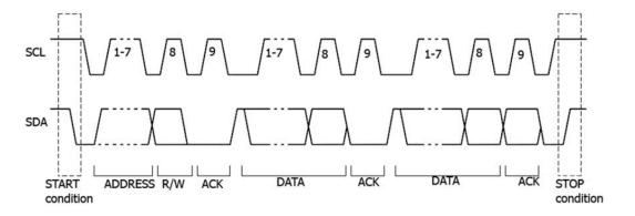
Figure 8.26 Schematic Diagram of I2C Protocol
