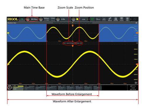
Figure 6.2 Delayed Sweep Mode
