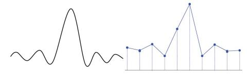
• **Waveform Aliasing:** when the sample rate is twice lower than the actual signal frequency (Nyquist Frequency), the frequency of the waveform rebuilt from the sample data is smaller than the actual signal frequency.
