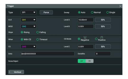
Figure 8.31 SPI Trigger Setting Menu
