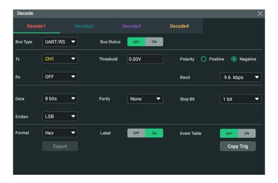
Figure 17.6 UART/RS232 Decoding Menu
