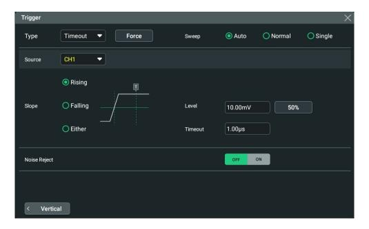
Figure 8.14 Timeout Trigger Menu
