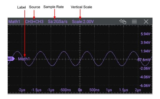
**Figure 9.4 Operation Result Display Window**
