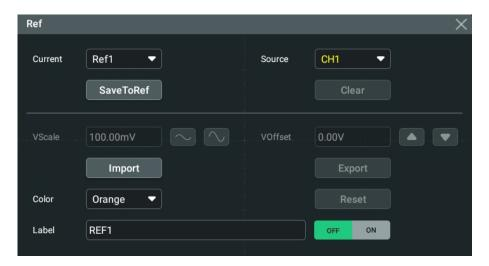
**Figure 15.1 Reference Waveform Menu**
