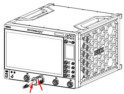
Active Probe Probe Adapter
