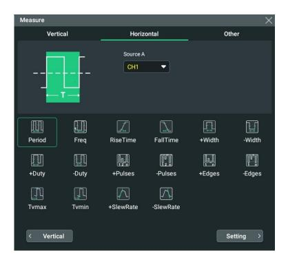
**Figure 10.5 Horizontal Measurement Items**
