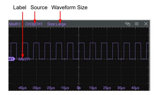
Figure 9.11 Operation Result Display Window
