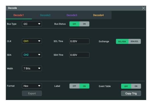
Figure 17.9 I2C Decoding Menu
