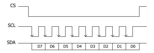
Figure 8.30 Sequential Chart of SPI Bus
