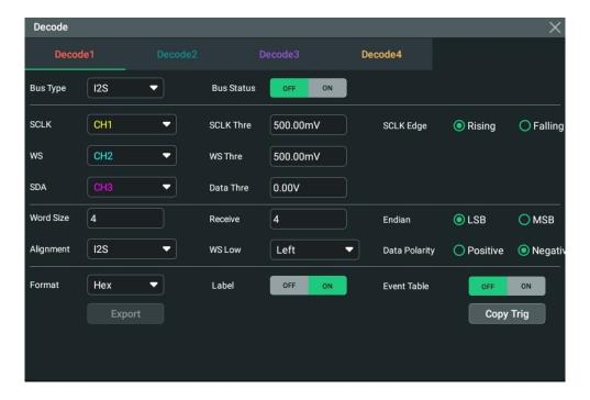
Figure 17.22 I2S Decoding Menu
