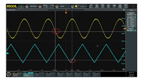
Figure 10.13 Track Measurement (before Horizontal Expansion)
