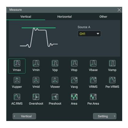
**Figure 10.4 Vertical Measurement Items**
