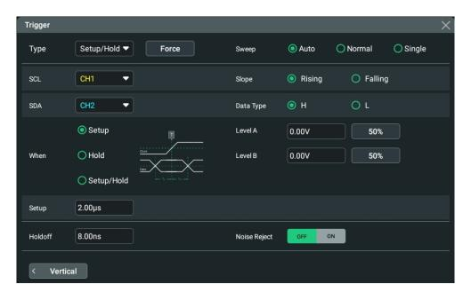
Figure 8.21 Setup/Hold Trigger Setting Menu
