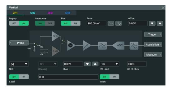
Figure 5.1 Vertical Menu for Channel
