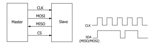
Figure 17.11 SPI Serial Bus
