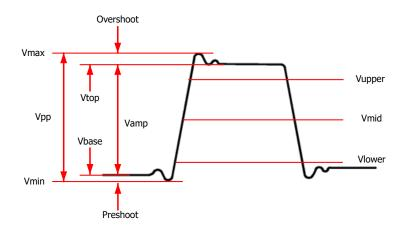
**Figure 10.3 Voltage Parameters**
