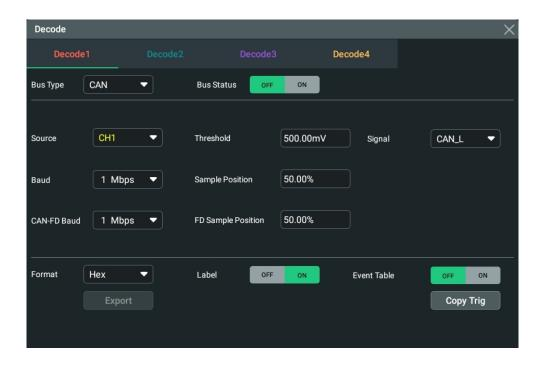
Figure 17.16 CAN Decoding Menu
