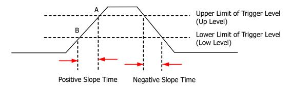
Figure 8.6 Positive Slope Time/Negative Slope Time
