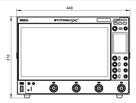
Figure 4.1 Front View (Unit: mm)
