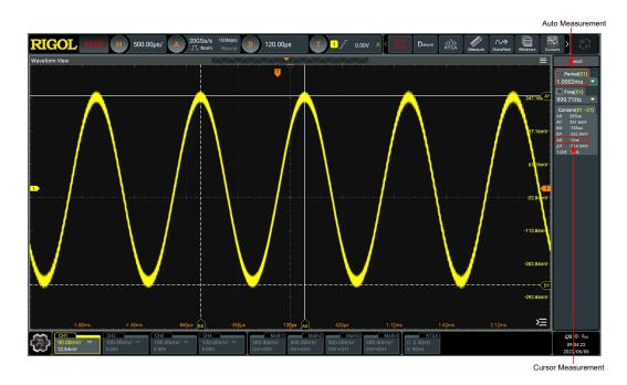
Figure 10.11 Manual Cursor Measurement Example
