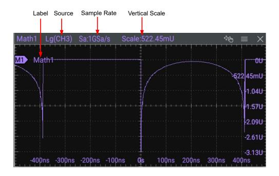
**Figure 9.6 Operation Result Display Window**
