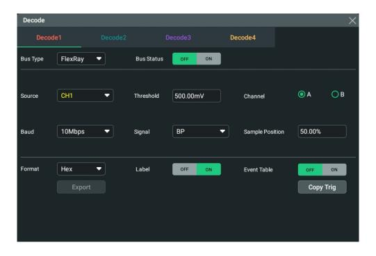
Figure 17.19 FlexRay Decoding Menu
