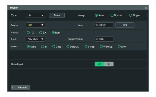
Figure 8.38 LIN Trigger Setting Menu
