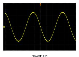
Figure 5.2 Waveform Invert
