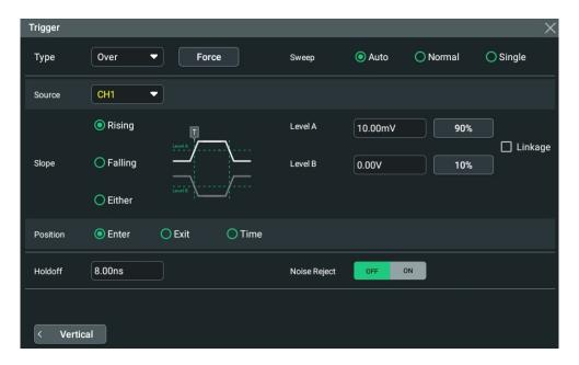
Figure 8.17 Window Trigger Setting Menu
